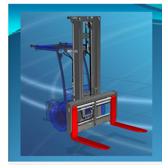
The market demand has led to the need of newly designed integral attachments with a more attractive look, which enable a better visibility by utilising fewer components and obtaining with less obstructions a much better view through the carriage.
